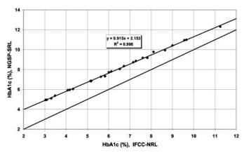
Fig. 1.  $HbA_{1c}$  values measured in 26 pooled blood samples by the IFCC-NRL, applying the IFCC Reference Method (mean value of 11 network laboratories), and by the NGSP-NRL, applying various methods adjusted to the NGSP DCM Bio-Rex 70 HPLC (mean values of 9 network laboratories).
